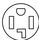
4-wire receptacle (14-30R)
