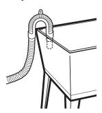
Use the provided tie strap to secure the drain hose in place.
