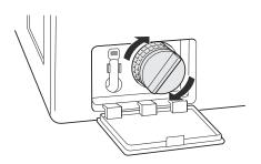
Close the drain pump filter cover.
