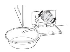
5 Clean the pump filter and opening.
