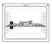
**2** If the level doesn't show that the rack is level, adjust the leveling legs with a wrench.
