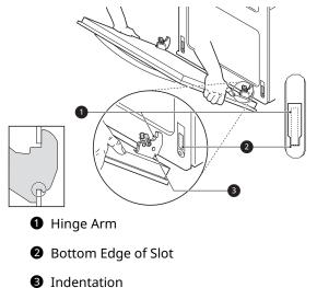
**3** Slowly open the door fully. Make sure that the hinge arms are properly engaged in the slots.
