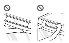
• Do not push or pull the range by grabbing the open oven door or cooktop only. Doing so can result in serious damage to the range.
