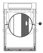
Secure the oven to the cabinet with screws provided. If the cabinet is particle board, you must use 3/4" particle board screws. These may be purchased at any hardware store.
