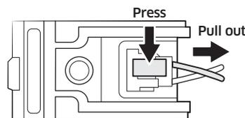
4. Press the hook of connector which is locked to the LED lamp board and pull out the wire connector.
