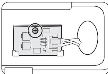
3. Remove the screw securing the LED lamp board.
