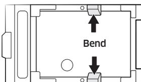
5. Remove LED lamp board by bending hooks which is holding it.
