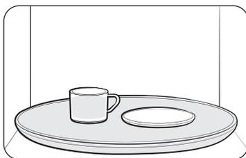
1. Fill a 1 cup glass measuring cup with water and put it inside your oven, next to the dish you want to test.
