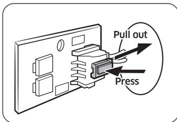
4. Disconnect the wire connectors by pressing the hook of connector which is locked to the LED lamp board.
