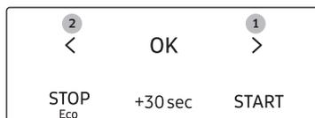
1. To add more cooking time during manual cooking mode, touch the '>' button. Each time you touch the '>' button, cooking time will be increased by 10 seconds.
