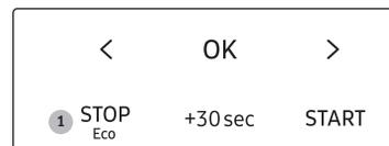
Eco Mode reduces standby power usage. When you touch the **STOP Eco** button once, the display will go out and the microwave shifts to a mode which minimizes power usage. To cancel the Eco mode, touch any button.
