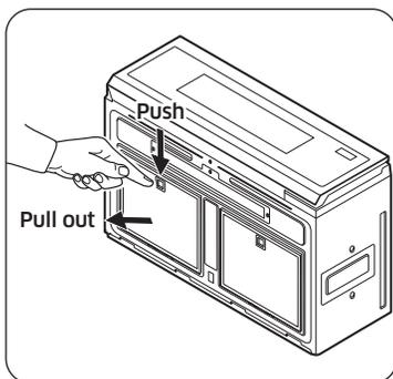
1. To remove the filter, push the handle of the grease filter.
