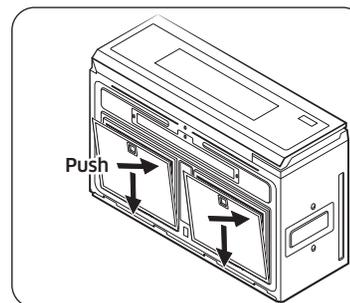
4. To re-insert the filter into the microwave oven, slide the filter into the frame slot, and then push it inside.
