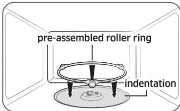
3. Install the pre-assembled ring into the indentation at the center of the microwave oven.
