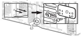
**5** Align the No. **6** bracket frame with the hole in the top of the product and assemble it using the No. **5** screw.
