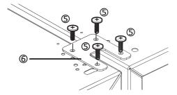
6 Remove the No. ⑤ screw from the bottom of the front of the product. Align the No. ② bracket frame with the hole in the product and reassemble it using the No. ⑤ screw.
