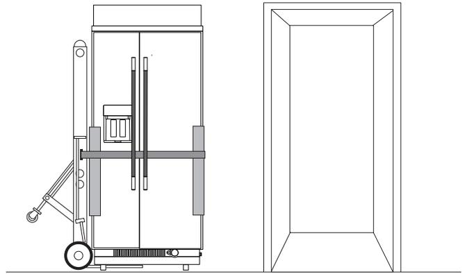
6. Place top of cardboard carton or plywood under refrigerator.
