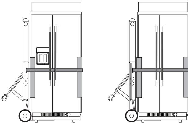
4. Place side pieces of the shipping carton in front of the cabinetry opening and on the floor when rolling the dolly into the house.
