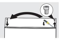
Remove the door and lay flat on a padded surface. Remove the door stop plate at the bottom of the door, and reinstall on the opposite side of door.
