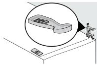
Remove the hinge pin from the right side hole and reinstall it on the left side hole on the top hinge using an adjustable wrench.
