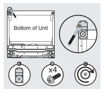
Carefully stand the freezer up. Place the door on the bottom hinge pin at 90° and rotate to the closed position.
