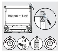
7. Unscrew and insert the hinge pin on the opposite side of the bottom hinge using an adjustable wrench.
