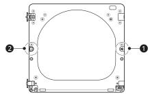
Remove the two screws on the door cover that secure the door strike. Remove the blank cover by pulling and raising.
