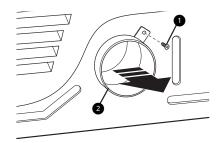
Press the tabs on the knockout 3 and carefully remove the knockout for the desired vent opening. (Right-side venting is not available on gas models.) Press the adapter
