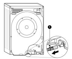
Connect the drain hose of the dryer and secure the hose clamp.
