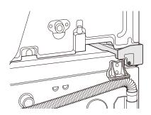
Insert the front bracket between the bottom of the appliance and the top of the washer. Push the front bracket toward the back of the washer until it comes in contact with the side bracket stoppers. Install the two remaining screws to secure the front bracket to the side brackets.
